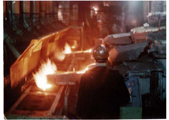
Dosing electromagnetic pouring of pig-iron on the automatic transfer line.
