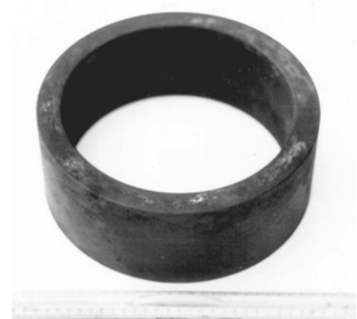
Casting obtained in sand mould for slider bearings used in 3M151 grinding machines and H483 guillotine scissors.
